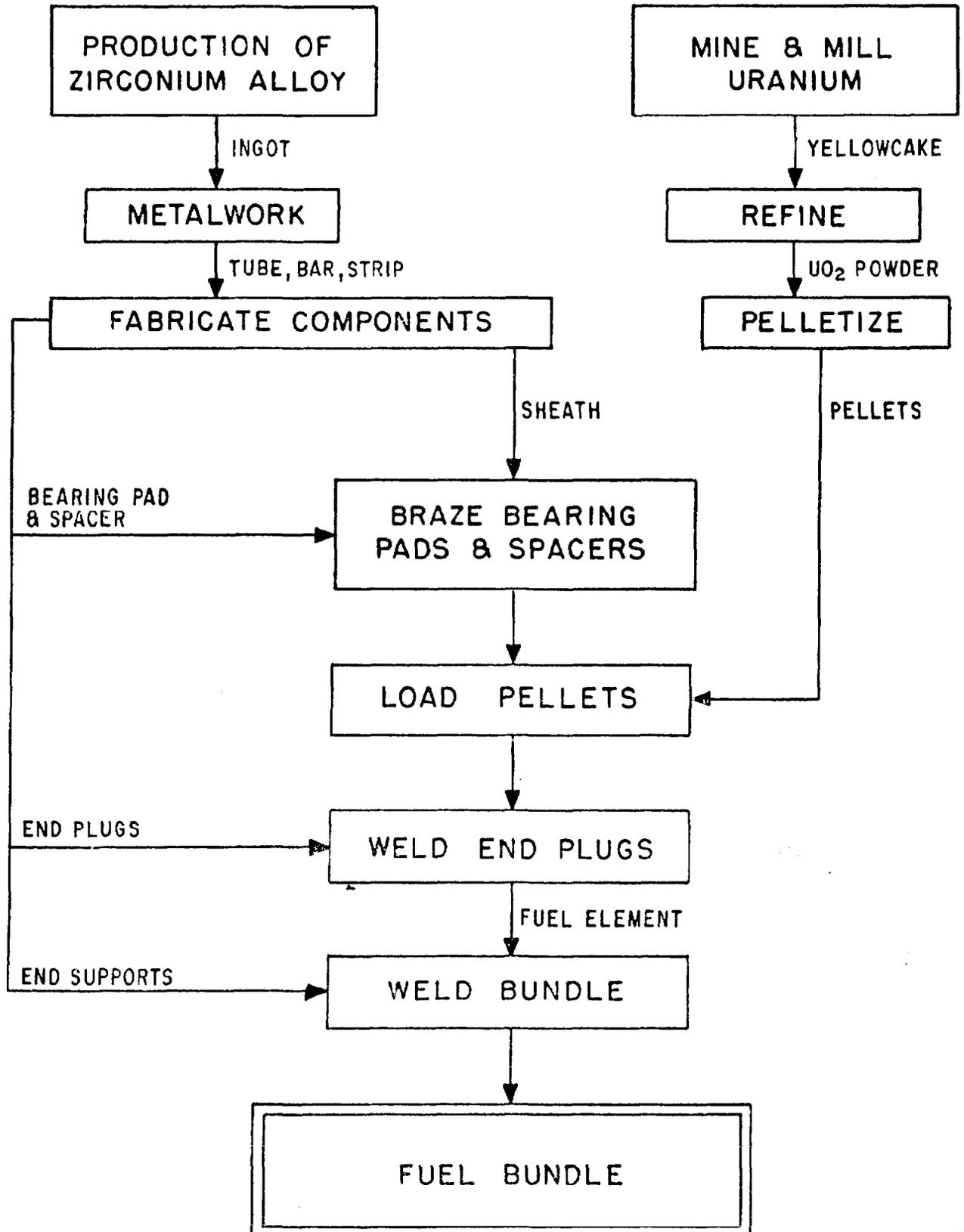
Earlier fuel used Zircaloy-2, the difference being the depletion of nickel content and increase of iron content in Zircaloy-4 which leads to performance advantages with respect to
